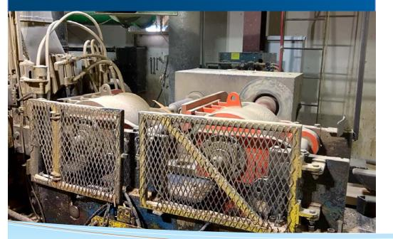
Combining superior control systems expertise & Bosch Rexroth innovations, AMS has developed an industry-leading, maintenance-friendly planer tensioning system. This system is proven to significantly reduce production downtime caused by planer jams, as well as mechanical maintenance & repairs.
